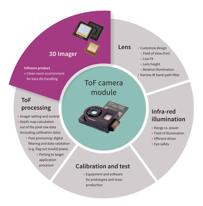
The basis for a 3D ToF module design is the REAL3™ imager, but to come to a complete 3D ToF module solution also other core components like lens and VCSEL as well as calibration expertise and depth processing software are required, everything optimized in a way to meet the application requirements.
