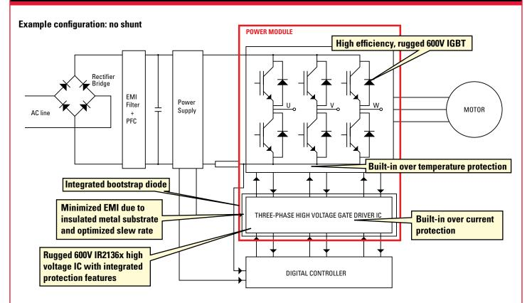
Built-in over-temperature/over-current protection, along with short-circuit rated IGBTs, an integrated under-voltage lockout function, and built-in temperature monitor provide a high level of protection and fail-safe operation. Other integrated features, such as bootstrap diodes for the high-side drive function and the single polarity power supply, simplify overall system design.
