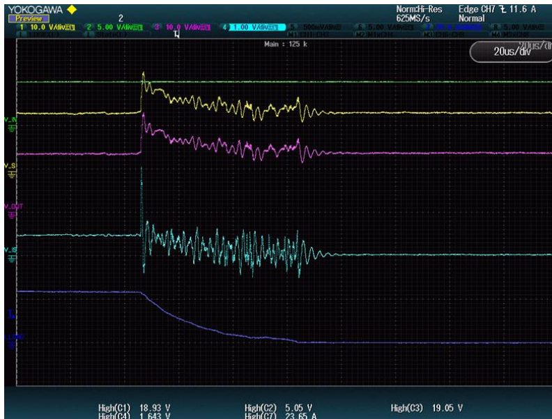
Figure 6 Loss of Load – BTS50010-1TAD scope plot example
