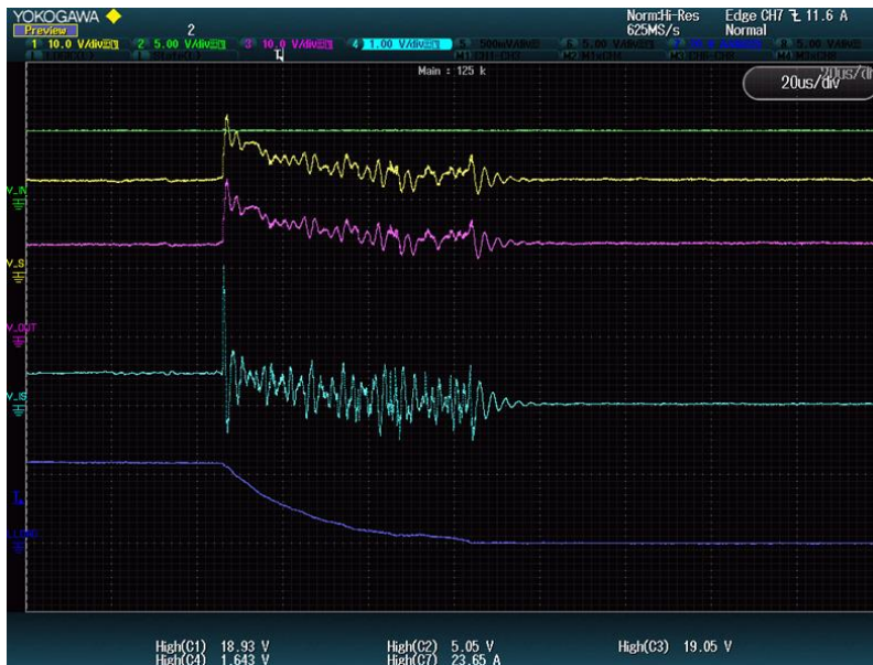
Figure 6 Loss of Load – BTS50010-1TAD scope plot example
