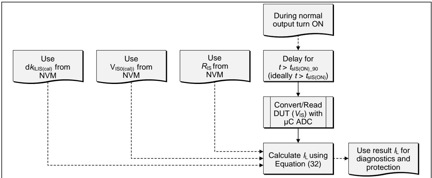
Figure 19 Application software procedure for the 2-Point calibration option
