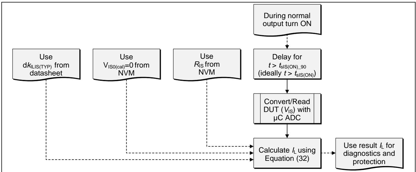
Figure 15 Application software procedure for No Calibration option
