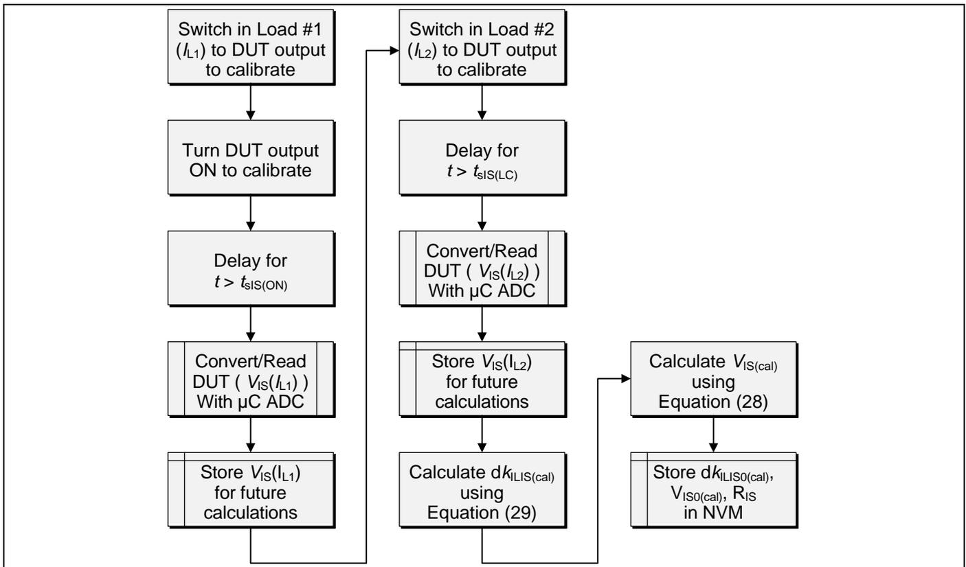
**Figure 18 Manufacturing test procedure for the 2-Point calibration option**
