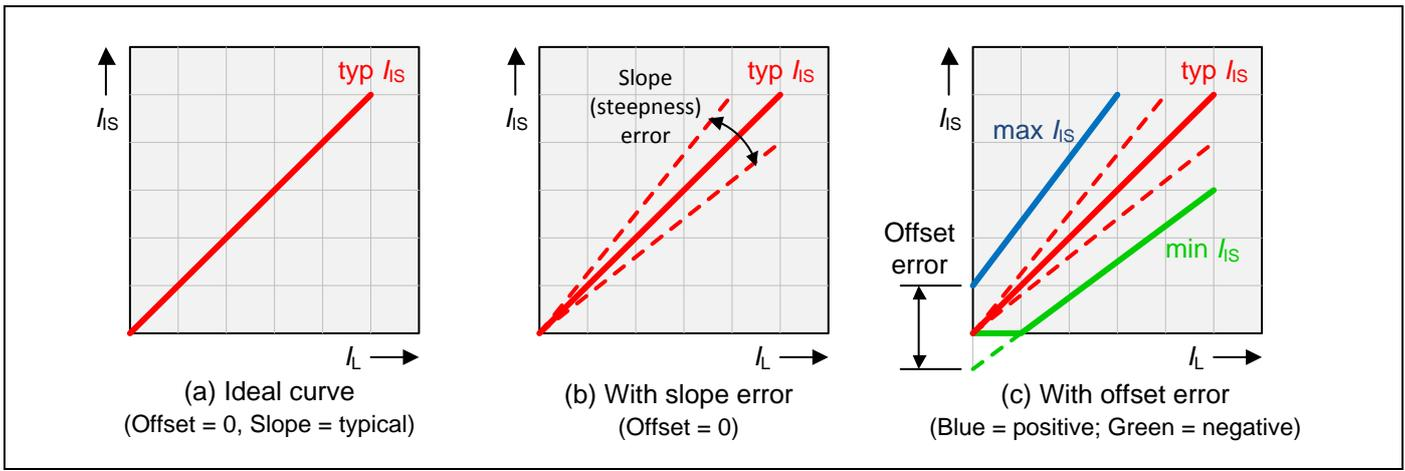
Figure 7 Relationship between  $I_s$  and  $I_L$  in conventional devices
