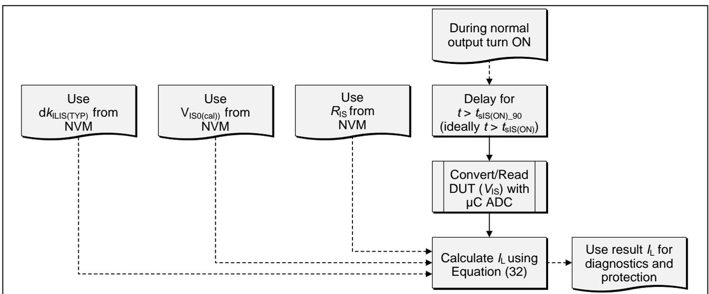
Figure 17 Application software procedure for the 1-point calibration option
