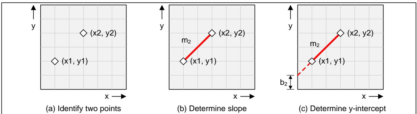
**Figure 12 Determining the characteristics of a straight line**
