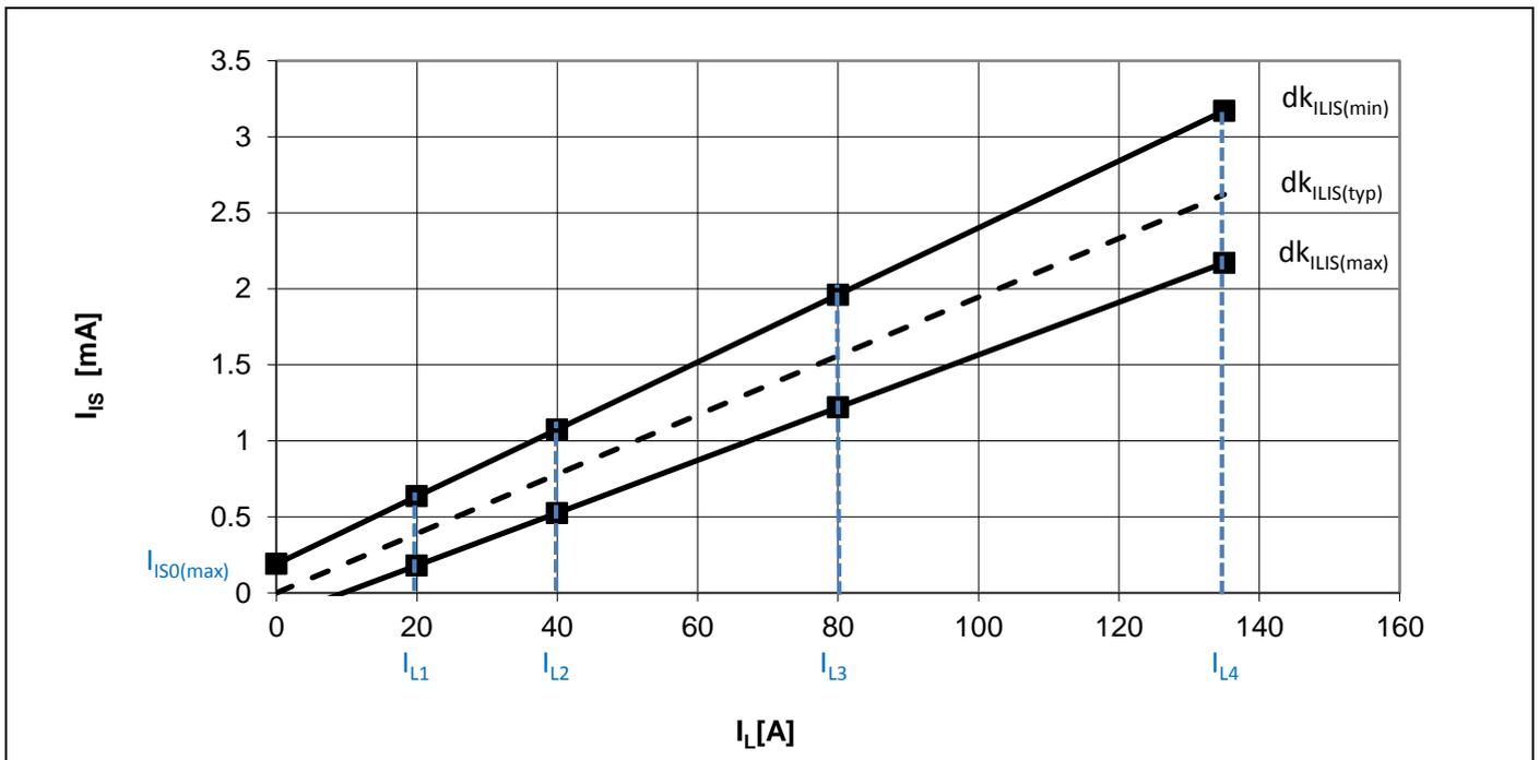
Figure 9 Power PROFET BTS50015-1TAD current sense
