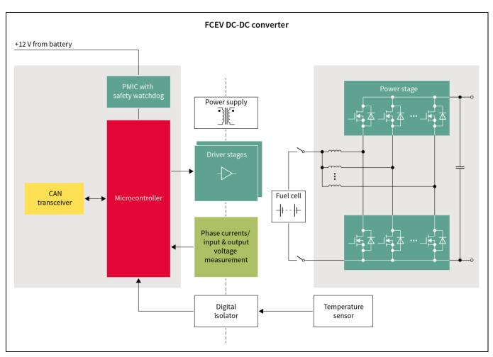
Figure 4 The DC-DC converter produces the DC link voltage from the fuel cell stack voltage
