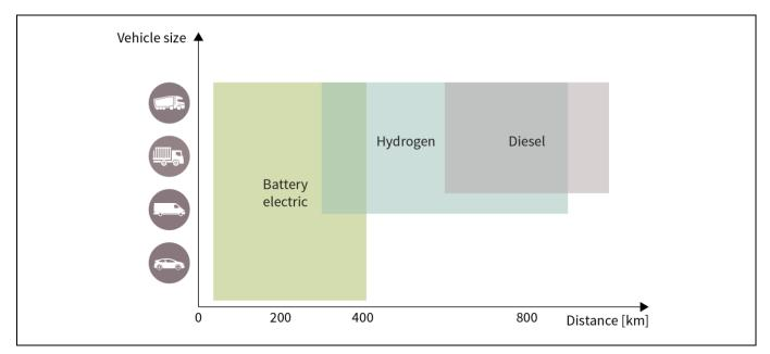
Figure 1 The size and range of the commercial vehicle will determine the drivetrain
