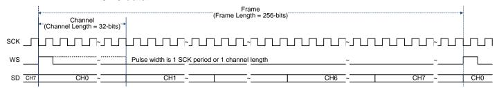
> TDM Mode B format: WS rising edge signal to signify that the start of frame is one-bit clock (SCK) early, relative to the start of CH0 data (coincides with the last bit of the previous frame)
