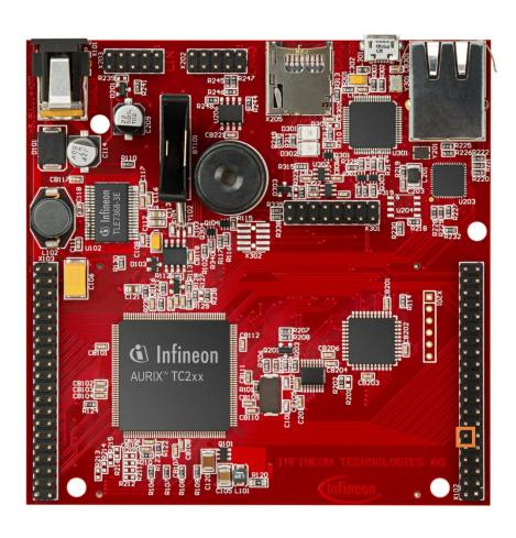
This code example has been developed for the board KIT\_AURIX\_TC297\_TFT\_BC-Step. The signal to be measured has to be connected to channel 0 of the VADC (port pin AN0).
