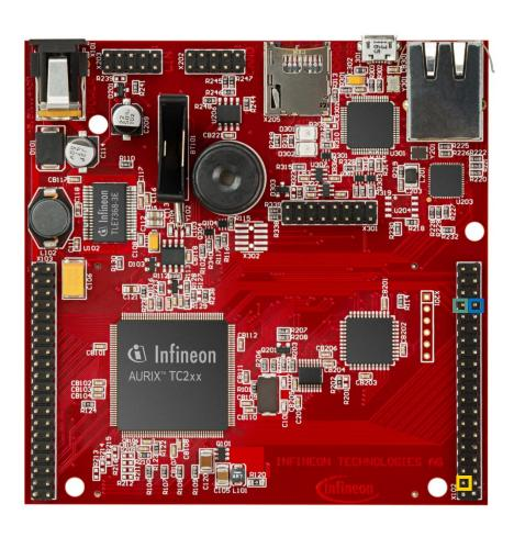
This code example has been developed for the board KIT\_AURIX\_TC297\_TFT\_BC-Step. The port pin P15.4 (SPI-MTSR) should be connected to the port pin P15.5 (SPI-MRST) in order to form an internal loopback. Those pins can also be connected to an
