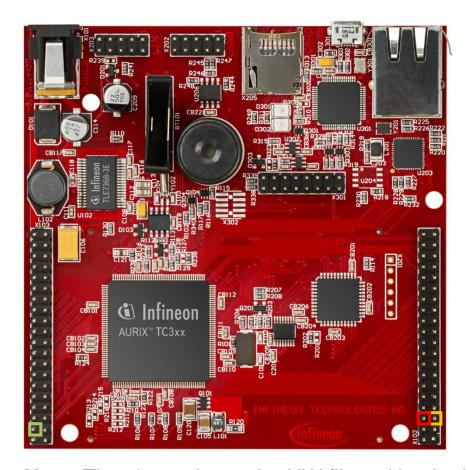
The signals to be measured have to be connected to channels 1, 4 and 5 of the group 2 of the EVADC (pins AN17, AN20, AN21).
