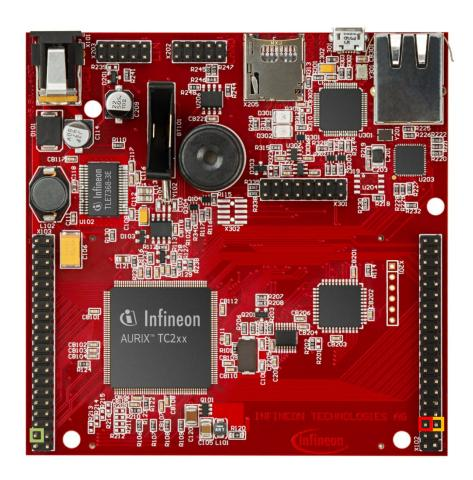
The signals to be measured have to be connected to channels 1, 4 and 5 of the group 2 of the VADC (pins AN17, AN20, AN21).
