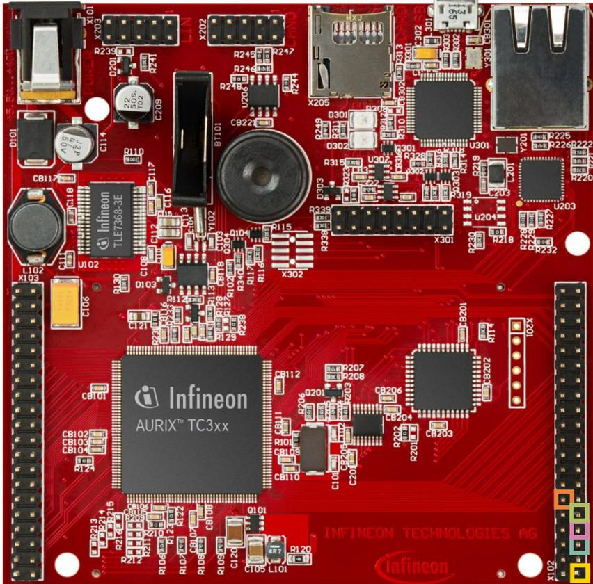
This code example has been developed for the board `KIT_A2G_TC397_5V_TFT`. In this example, the port pins `AN0`, `AN3`, `AN13` and `AN21` are used, connected to `VCC_IN`. For using the `VCC_IN`, the resistor `R113` must be soldered.
