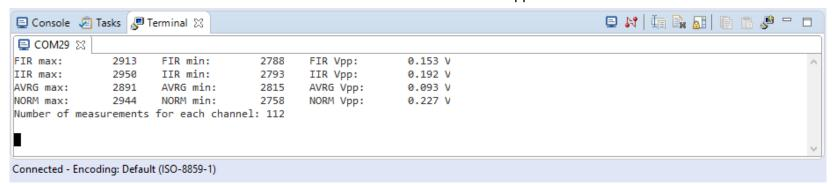
The maximum and minimum values are expressed as a 12-bits integer value, in decimal format (0 - 4095 range), while the  $V_{pp}$  is expressed in Volts
