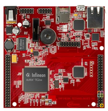
This code example has been developed for the board KIT\_AURIX\_TC297\_TFT\_BC-Step. In this example, the port pins AN0, AN2, AN3 and AN8 are used, connected to
