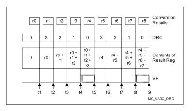
When the conversion is ready, depending on the configuration of the DRCTR bit field, the result register contains the sum of up to 4 result values, thus it is needed to divide the content of the result register GxRESy by the number of the accumulated values in order to obtain an average of the measurements.
