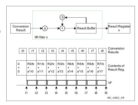
**Note:** In this example, a delay before starting to read the conversion results is needed. This ensures that reading spikes in the VCC\_IN supply due to the initialization of the device are avoided and that incorrect values are not read due to the filters not being yet at full speed.
