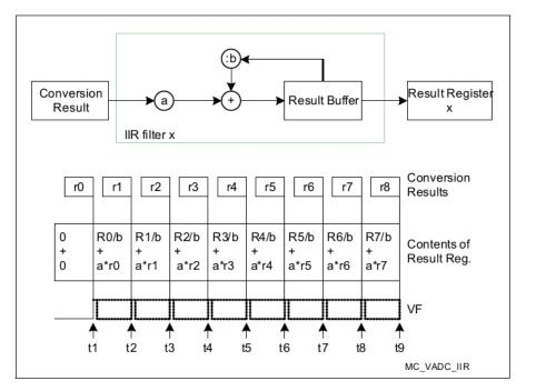
**Note:** In this example, a delay before starting to read the conversion results is needed. This ensures that incorrect values are not read due to the filters not being yet at full speed.
