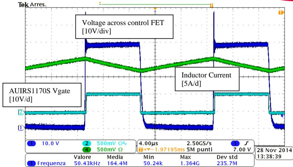
Figure 6: Positive-tied Buck converter waveforms
