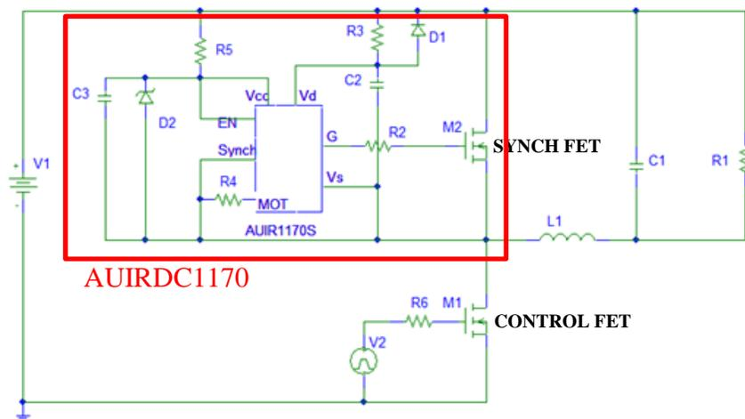
**Figure 5: the positive-tied synch. Buck converter test schematic**
