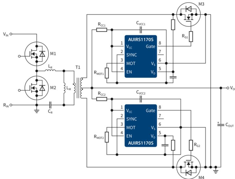
Figure 1: typical application diagram of the AUIRS1170S in a HV-DC/DC converter
