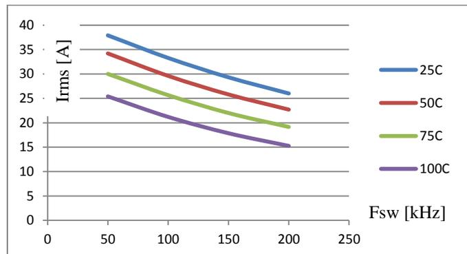
Figure 4:  $I_{RMS}$  rating vs  $T_{amb}$  and  $F_{sw}$
