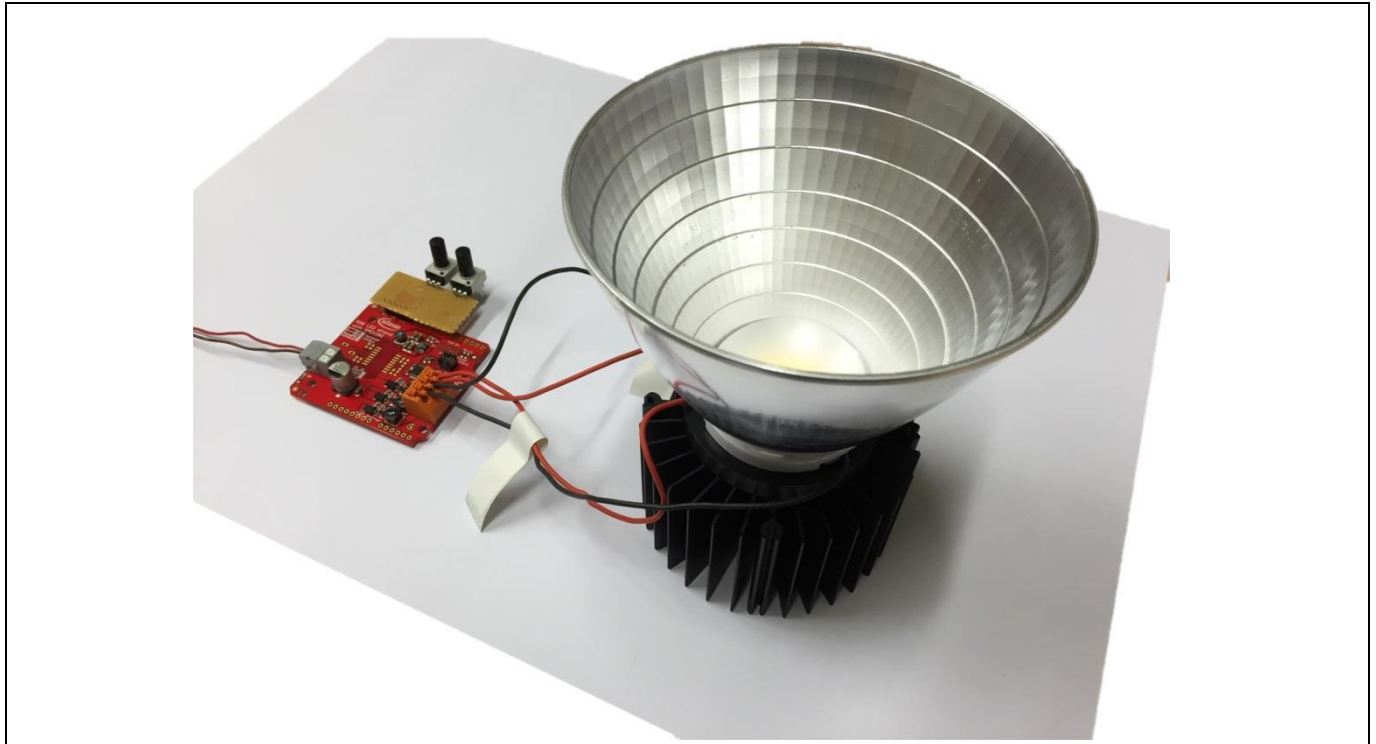
Figure 2 Modified RGB LED lighting shield for controlling tunable white LED lamp (in picture: Everlight's CHI3030)
