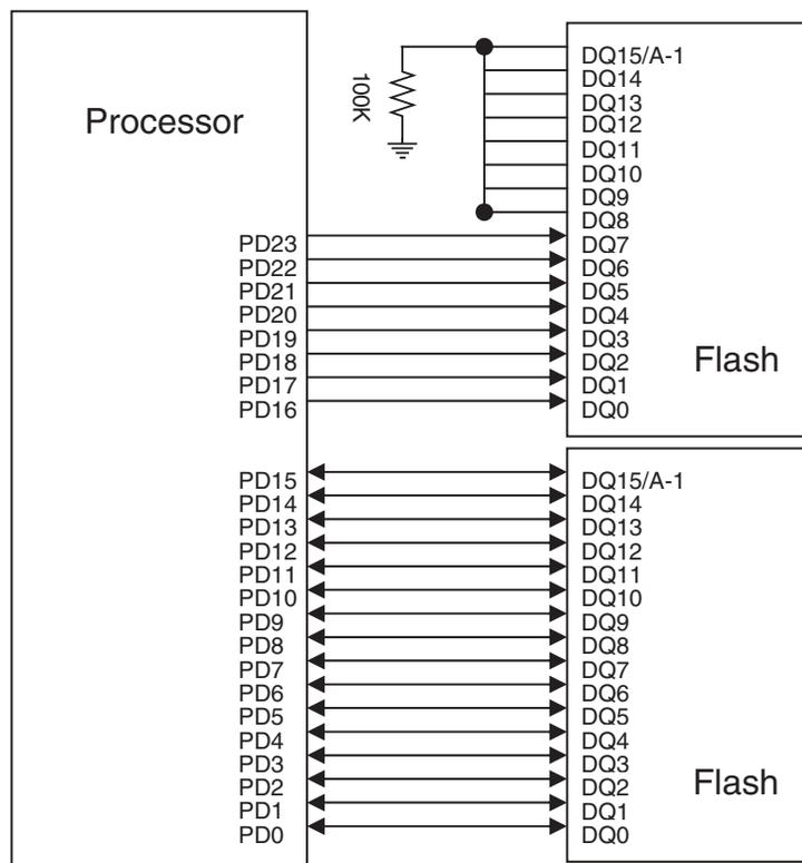
Note that on [Figure 1](#) the unused data pins on the Flash device of the upper word lane are pulled-down to ground through an external resistor (100 K $\Omega$  is recommended). Handling unused data lines in this manner is necessary for successful write buffer programming.
