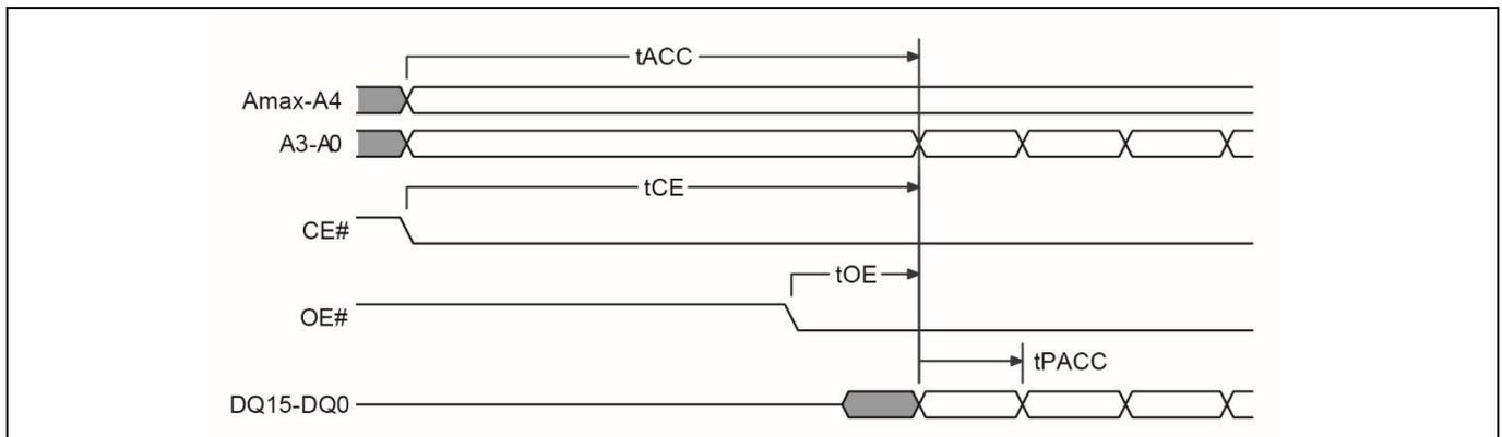
**Figure 6 S29GL-S Asynchronous / Page Read Access**
