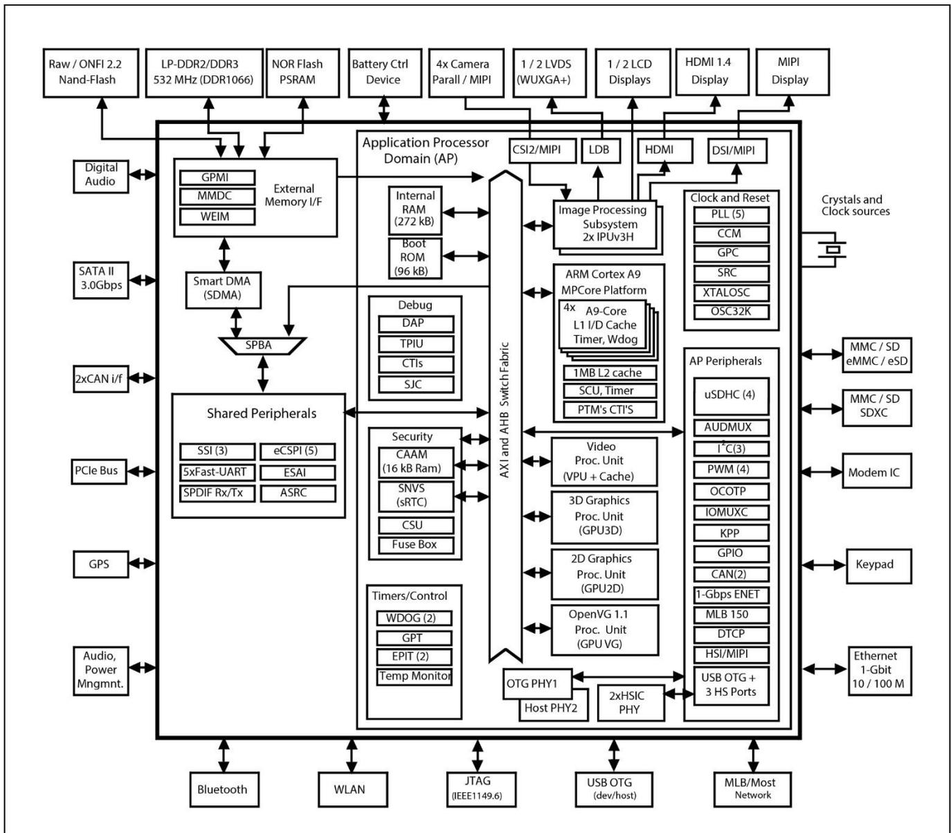
**Figure 1 i.MX6x Block Diagram**
