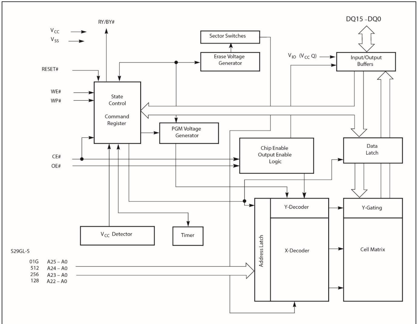
**Figure 3 S29GL Asynchronous / Page Mode Block Diagram**
