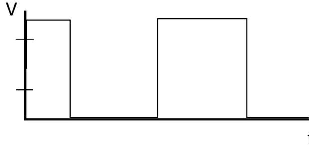
A nice thing about digital signals is, the system only needs to detect whether the voltage is in the “1” range or the “0” range. Depending on the system, a logic range can be fairly large and the signal can have a fair amount of distortion without obscuring the intended logic level or bit-state as shown in [Figure 2](#). Note such signal overshoot may directly or indirectly couple to power and ground planes thus affecting the fidelity of a subject ICs power system.
