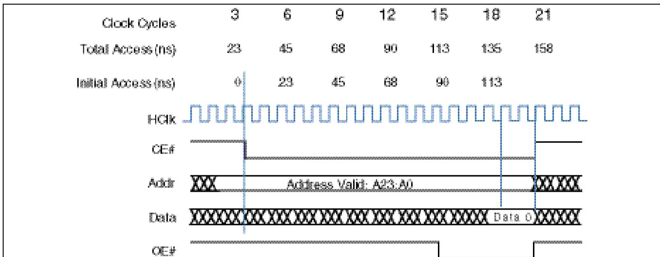
**Figure 1 iMX5x/S29GL256S Asynchronous read timing (1 Word)**
