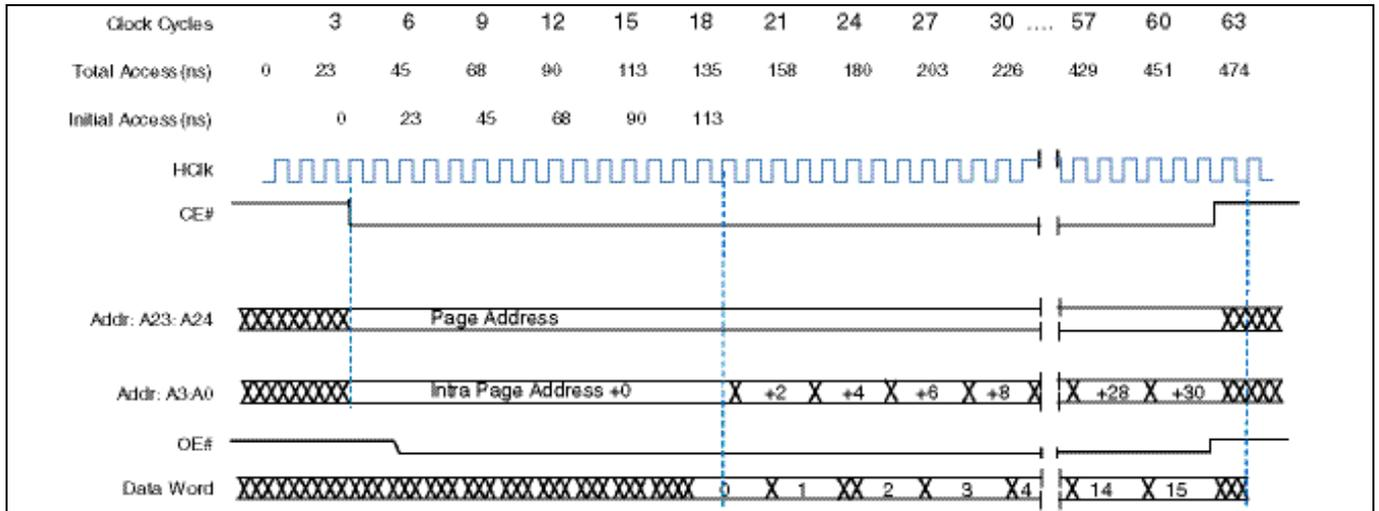
**Figure 2 iMX5x/S29GL256S page read timing (16 Words/32 Bytes)**
