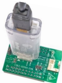
Figure 121. CYBLE-022001-EVAL Using CY8CKIT-002 MiniProg3
