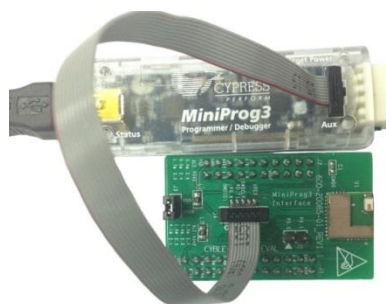
Figure 127. CYBLE-222014-EVAL Using CY8CKIT-002 MiniProg3
