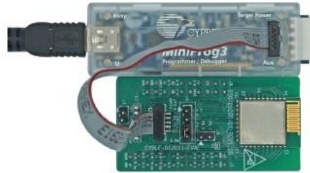
Figure 133. CYBLE-212019-EVAL Using CY8CKIT-002 MiniProg3 and 10-Pin Ribbon Cable
