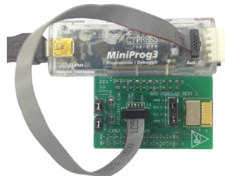
Figure 145. CYBLE-214015-EVAL Using CY8CKIT-002 MiniProg3 and 10-Pin Ribbon Cable
