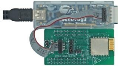
Figure 130. CYBLE-012011-EVAL Using CY8CKIT-002 MiniProg3 and 10-Pin Ribbon Cable
