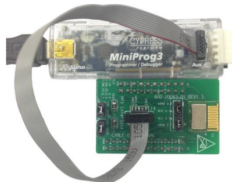
Figure 142. CYBLE-214009-EVAL Using CY8CKIT-002 MiniProg3 and 10-Pin Ribbon Cable
