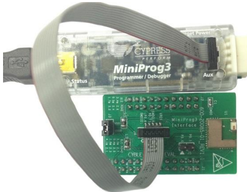
Figure 124. CYBLE-222005-EVAL Using CY8CKIT-002 MiniProg3
