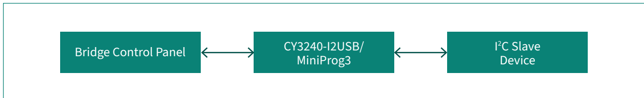
Figure 5-21 Bridge Control Panel Communication with I 2 C Slave Device
