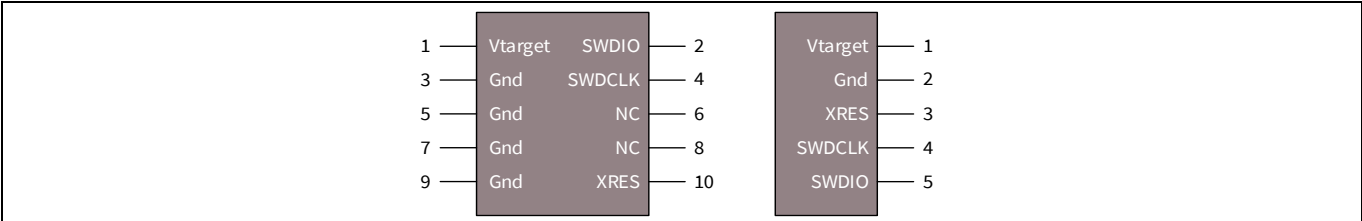
Figure 8 SWD connector pin maps for MiniProg3 or MiniProg4
