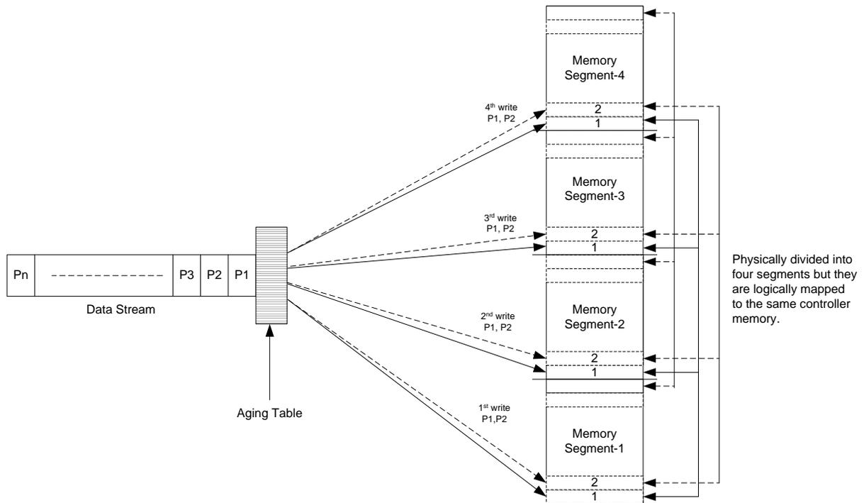
Wear leveling requires a fairly sophisticated driver routine in the controller, through which all nonvolatile accesses are managed. This routine translates the internal addressing of data structures into a physical addressing scheme for the memory. Usually, an “aging table” on the memory array tracks how the device is being used. This consumes a significant amount of code space in a miniature filing system.
