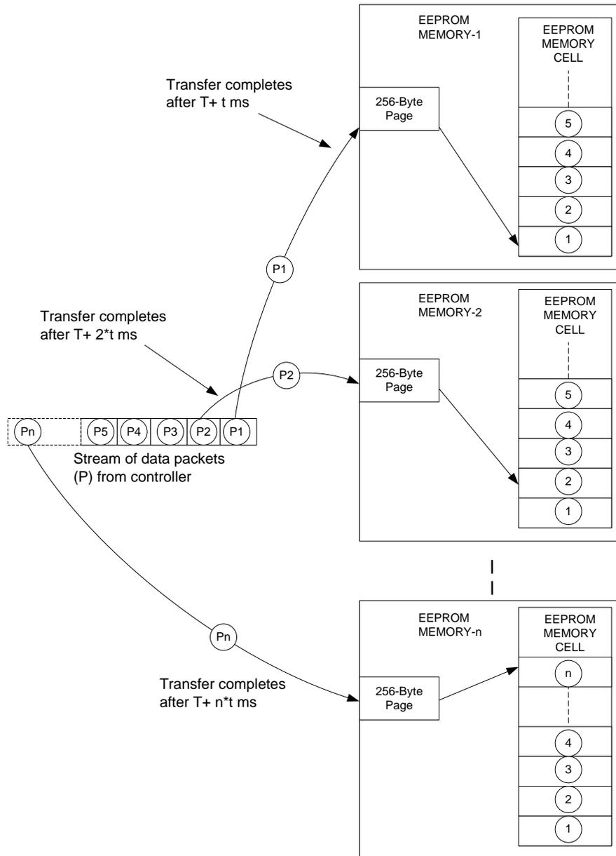
An I<sup>2</sup>C EEPROM interface with a 1-MHz access speed takes 2 ms to transfer 256 bytes (1 page) of data and 5 ms to complete the nonvolatile write cycle for each page. Therefore, a three-stage pipeline implementation is required to achieve the write to EEPROM at the bus speed.
