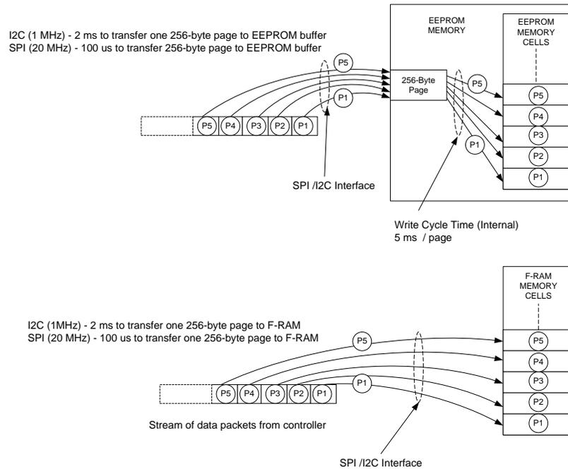
In addition, EEPROM supports varying page sizes; in this example, the lower page size in EEPROM requires more page write operations and more write cycle time. The result is additional write delays. Because F-RAM is not paged memory, the time to write a given set of data to it remains the same across all memory density options.
