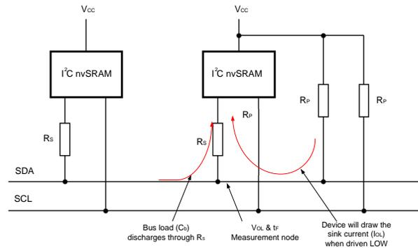
If series resistors are used, the additional resistance should be taken into the calculations for  $R_p$  and the allowable bus capacitance. In addition, the series resistance ( $R_s$ ) will increase the net output voltage level to a higher level ( $V_{OL} + R_s \times I_{OL}$ ), which will effectively reduce the noise margin at the receiving device end. The output fall time delay due to the additional  $R_s$  can be calculated using Equation 3:
