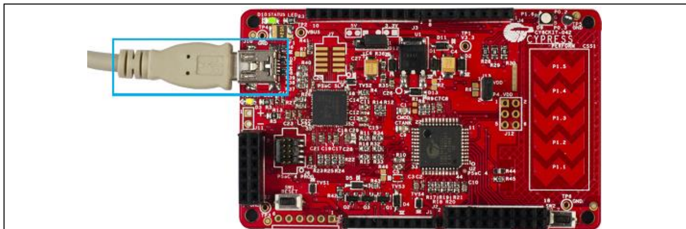
Figure 19 Connect USB Cable to J10 in CY8CKIT-042
