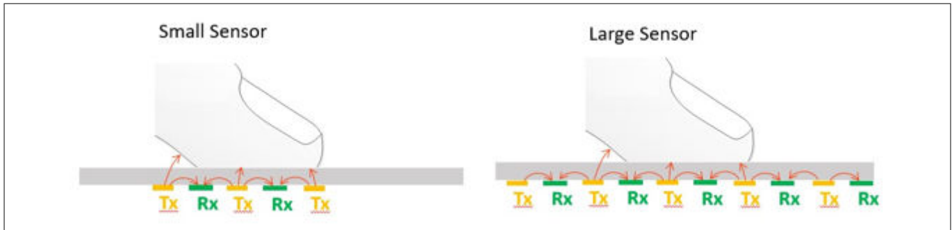
Figure 132 Interaction of electric field with the finger
