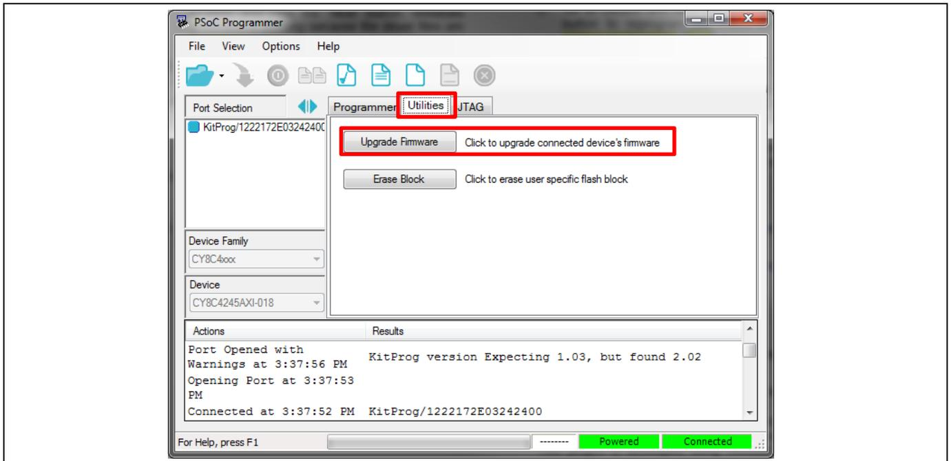
Figure 9 Upgrade Firmware using PSoC Programmer
