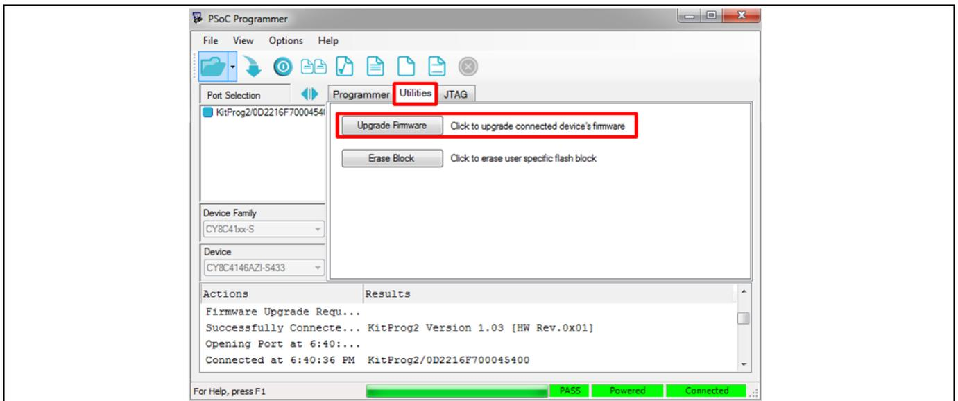
**Figure 14 Upgrade Firmware using PSoC Programmer**
