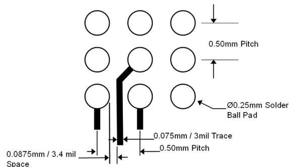
0.075-mm traces should only be used in BGA areas that have routing space constraints. Necking down traces can be used to increase manufacturability and ensure better yields. After the trace exits the BGA land pads, return to standard trace and space geometry as shown in [Figure 10](#).
