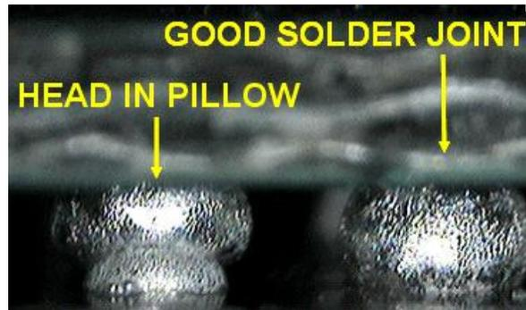
Head-in-pillow is a solder joint defect where the solder paste wets to the PCB land pad, but does not fully wet to the BGA solder ball. Although mechanical contact is made between the land pad and the BGA solder ball, the solder joint is not formed at a metallurgical level as shown in [Figure 15](#).
