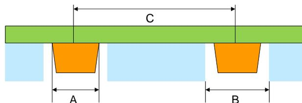
Table 4: BGA NSMD Solder Ball Pad Design (mm)
