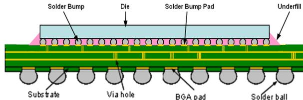
Wafer bumping is an essential process in flip chip packaging. The bumping process is an advanced packaging technique where bumps made of solder are formed on the wafers before being cut into the individual die.
