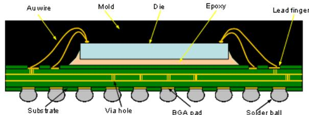
The standard BGA packaging process begins by dispensing epoxy on the substrate where the die is to be attached. For more advanced substrate designs, an adhesive film is laminated to the back of the wafer instead of using die attach epoxy. Next, a pretested die is picked from a wafer that has been cut and mounted on a tape ring, and placed on the substrate. A UV or oven cure hardens the epoxy/film material before wire-bonding the die to the substrate.
