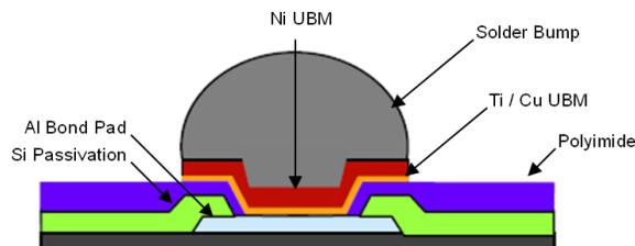
The flip chip BGA packaging process begins by dispensing flux on the substrate pads where the die is to be attached. Next, the bumped and pretested die is picked from a wafer that has been cut and mounted on a tape ring and placed on the substrate. The solder bumped die is attached to the substrate by a solder reflow process very similar to the process used to attach BGA balls to a PCB.
