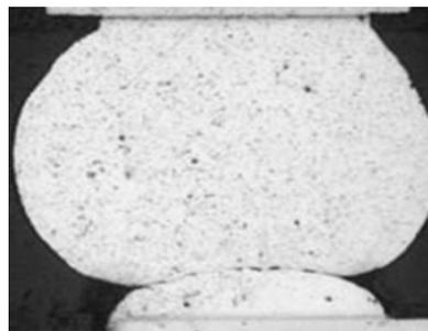
Because the solder joint lacks strength, components with head-in-pillow defects may fail with very little mechanical or thermal stress. Unfortunately, this defect is usually not found during functional testing but rather in the field after the assembly is exposed to physical or thermal stress.
