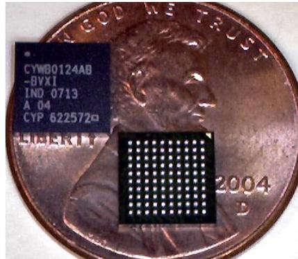
BGA packages provide a shorter conductor path between the die and the PCB/FPC because they use a substrate instead of a lead frame. The shorter path provides lower inductance, which results in better electrical performance, minimizing signal distortion in high-speed applications. The substrate also provides better heat dissipation by allowing the heat generated by the device to flow from the back of the die, through the solder balls, and to the PCB/FPC.
