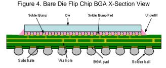
Wafer bumping is an essential process in flip chip packaging. The bumping process is an advanced packaging technique where bumps made of solder are formed on the wafers before being cut into the individual die.
