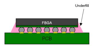
Figure 17. BGA Mounted to a PCB with Underfill
