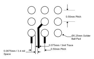
Figure 9. Signal Line Space and Trace Width
