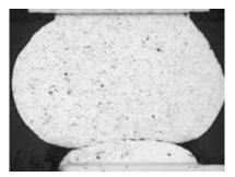
Because the solder joint lacks strength, components with head-in-pillow defects may fail with very little mechanical or thermal stress. Unfortunately, this defect is usually not found during functional testing but rather in the field after the assembly is exposed to physical or thermal stress.
