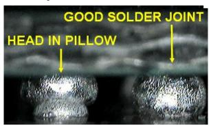
Figure 14. Post Reflow Solder Joints
