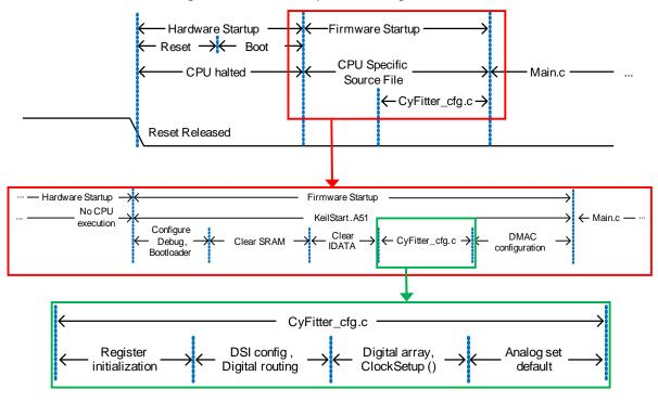
Figure 26. Device Startup Process Diagrams
