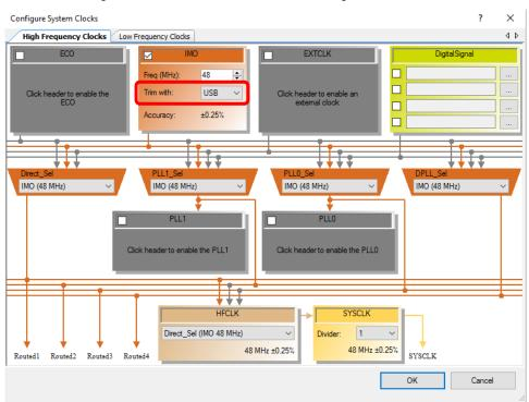
Figure 7. PSoC 4 L-series USB Clock Configuration
