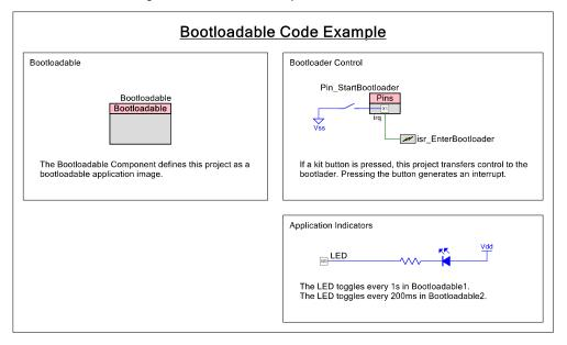
Figure 9. Bootloadable Project Schematic
