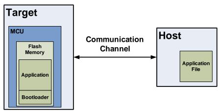
Typically, the system that provides the data to update the flash is called the **host**, and the system being updated is called the **target**. The host can be an external PC or another MCU on the same PCB as the target.
