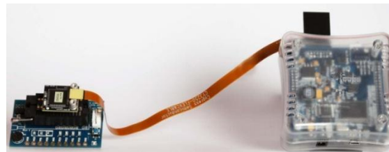
Figure 15. ICE Connected to CY3250 Pod
