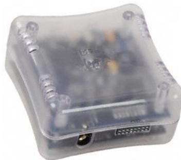
Figure 4. In-Circuit Emulator (ICE)
