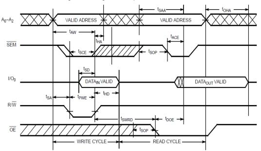
Figure 5. Timing of a Semaphore Read After a Write
