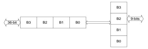
Figure 10. Little-Endian Byte Mapping Between 18-Bit and 9-Bit Buses
