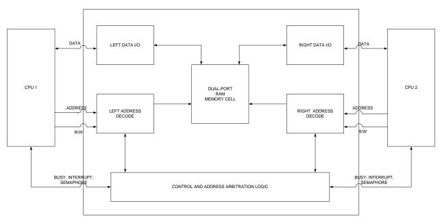
Figure 11. Processor Communication with Dual-Port Shared Memory
