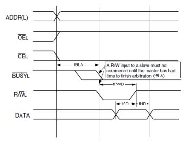
Figure 7. Timing Required for Width Expansion
