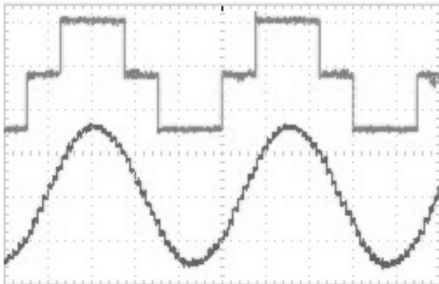
That's a nice clean sine wave although the 40 samples per cycle transitions can be clearly seen.
