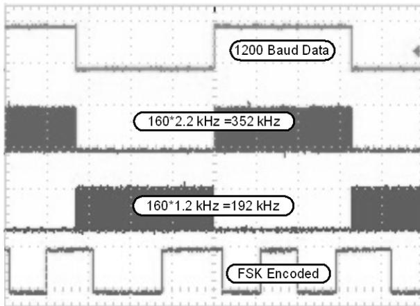
The HART modem spec allows up to 20 degrees phase error in the transition from one bit to the next. Since the output frequency is derived from a 160x clock, the phase error will be between 0 and 2.25 degrees. This exceptionally clean phase transition limits the inter-symbol error and enables easier detection of the FSK data at the receiving end. What remains is turning that square wave into a respectable sine wave, or something with low enough harmonics to meet the intent of the spec.
