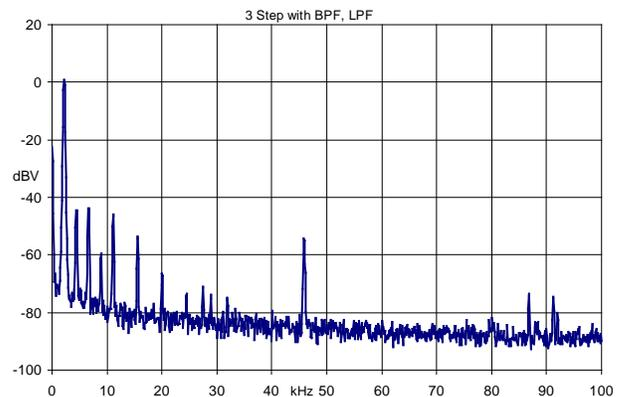
The highest harmonic is the third at -44 dB, the total distortion is less than 0.8; the highest alias is at 998 kHz at -52 dB; this is a very clean, easily generated waveform.
