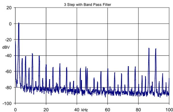
The harmonics of Figure 8 are considerably reduced from the levels shown in Figure 5. The highest harmonic is the fifth at 38.5 dB below carrier, or 1.1% of distortion. All others are lower except the lines at 87.8 and 90.2 kHz; these are the sampling aliases of the filter with a level 32 dB below carrier. The sum of the low-order harmonics and the first pair of aliases results in a signal to noise ratio of 29 dB or 3.3% distortion.
