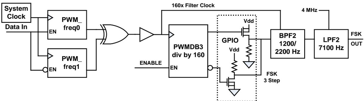
Design of the band pass filter is enabled by using either the filter wizard in PSoC Designer™ or the design spreadsheet in PSoC Designer→Help→Documentation. The input to the filter is a 5.0 Vpp signal, which is large enough to saturate the filter output unless the filter is designed to attenuate the signal. Narrow band PSoC filters have high gain, this is a mathematical limitation based on the range of capacitor values available.
