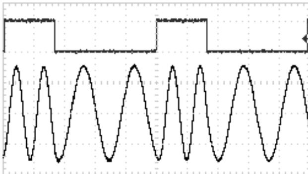
The design is demonstrated at 1200 Hz and 2200 Hz, Bell 202 standard 1200 baud modem frequencies. Common applications for these operating frequencies include telephone caller ID and Highway Addressable Receiver Transmitter (HART) modems. HART modems are used for transmission over DC power lines, often shared with 4-20 mA current loop data. The HART standard waveform, while not enforcing a specific requirement, has a relatively low distortion level. A simple square wave will not do.
