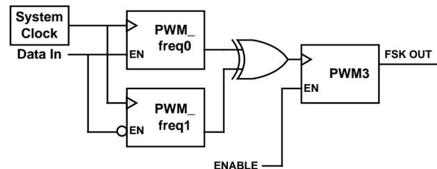
PWM\_freq1 divides the clock source to provide a fixed multiple of the output frequency at the logical 1 frequency,  $160 \times 2200$  Hz, or 352 kHz
