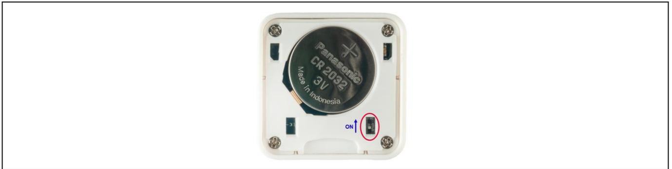
**Figure 2 Turn ON the sensor**
