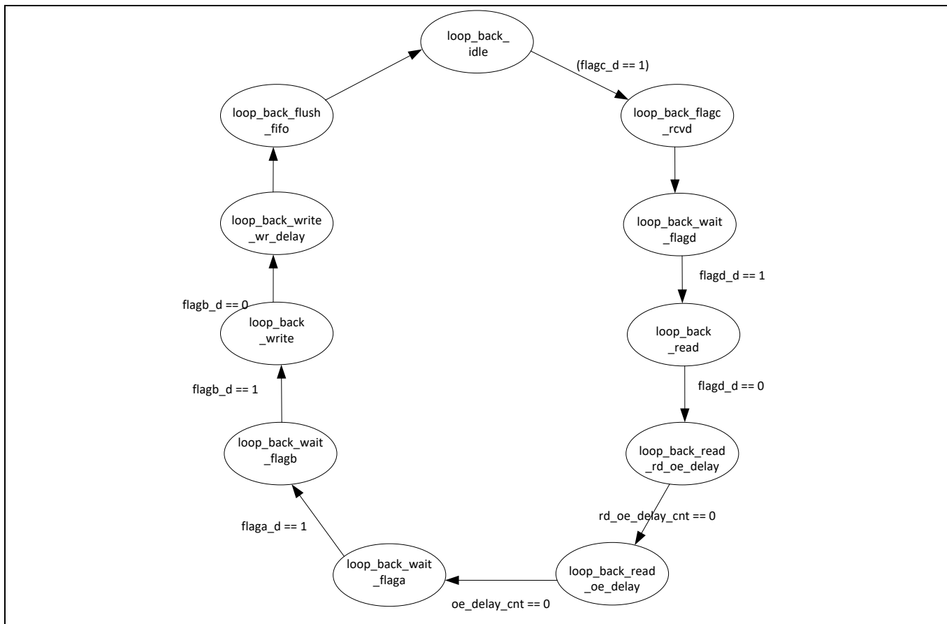
Figure 49 State machine for loopback transfer
