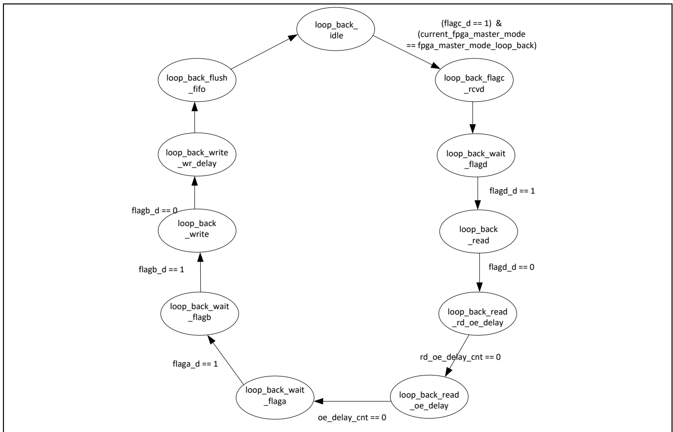
Figure 27 State machine for loopback transfer
