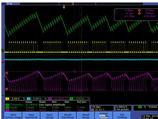
Figure 4 shows the operation of the circuit captured from a real system. The green waveform at the top is the inductor current. The magenta signal at the bottom is the load current. The yellow signal is the FET gate drive signal. The blue signal is the input voltage.
