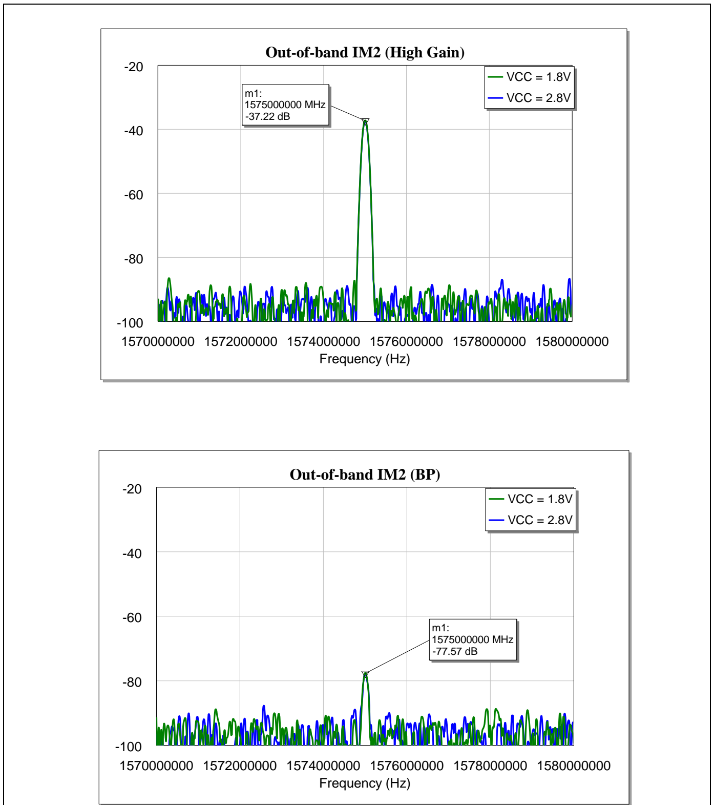
Figure 16 Out-of-band second-order intermodulation point of BGA5M1BN6 for GNSS applications (L1 band, power at input: -28 dBm, f1 = 827 MHz, f2 = 2402 MHz, output referred)
