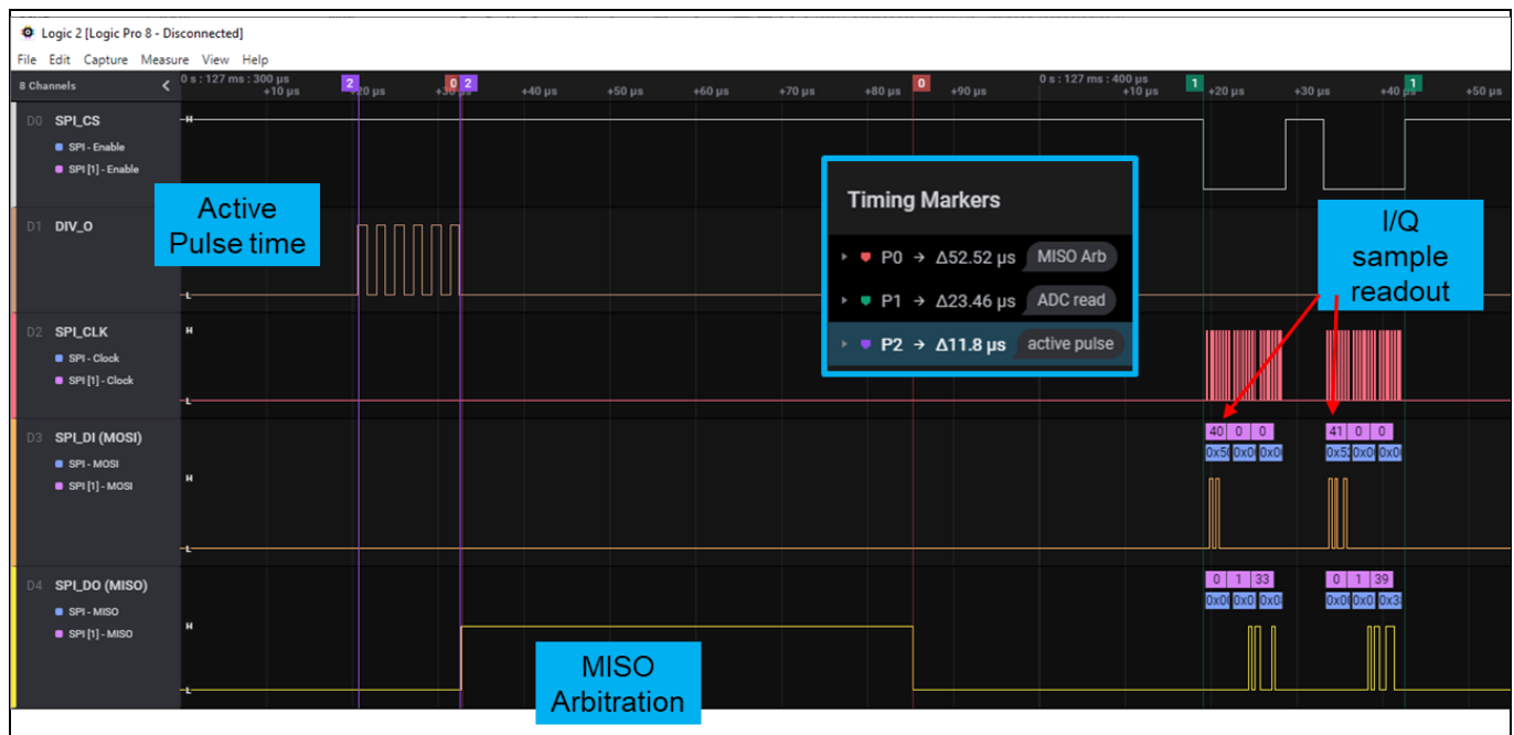
Figure 24 Typical SPI access
