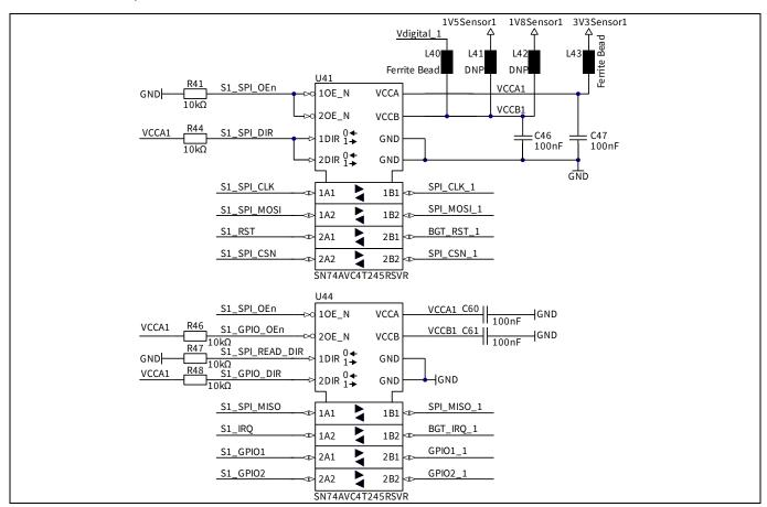
Figure 6 Level shifter circuit of sensor 1
