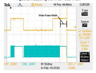
Figure 2. Measuring the Write Pulse Width
