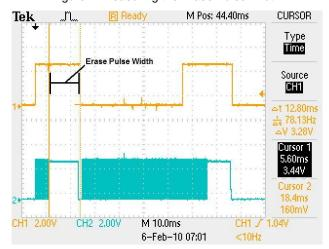
Figure 1. Measuring the Erase Pulse Width
