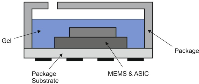
**Figure 1 DPS368 package drawing**
