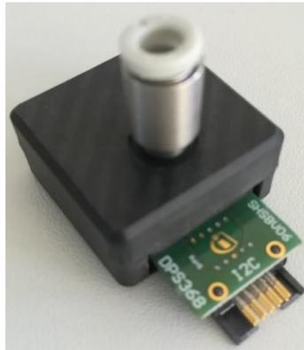
**Figure 8 Water-resistant evaluation board**
