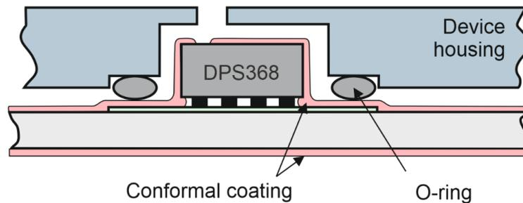
**Figure 5 System Integration with O-ring sealing and conformal PCB coating**
