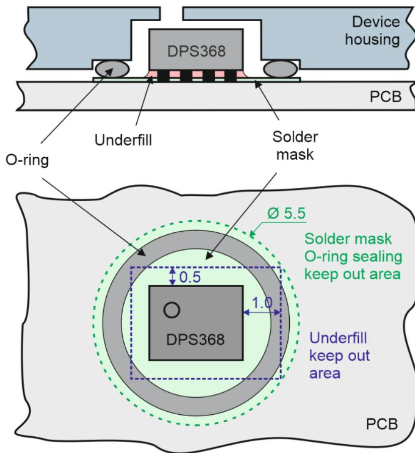
**Figure 3 System Integration with O-ring sealing and underfill**
