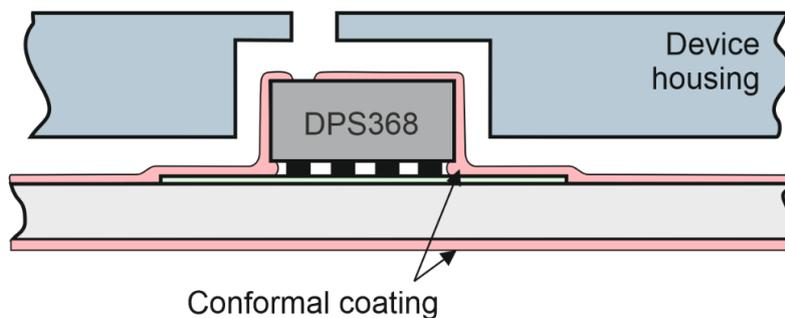
**Figure 6 System Integration with conformal PCB coating**
