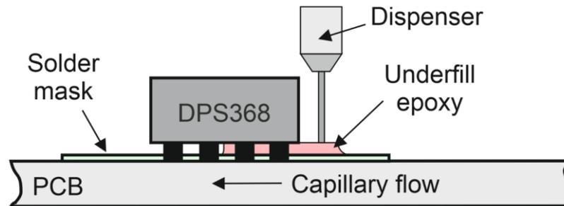
**Figure 4 Underfill application**
