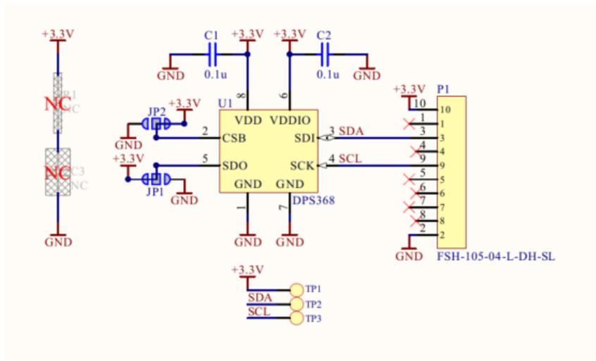
**Figure 9 Figure 9. Water-resistant evaluation board schematic**
