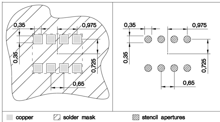
**Figure 2 PCB pad and stencil aperture recommendations**
