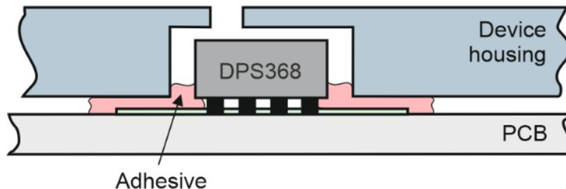
**Figure 7 System Integration using adhesive gel**
