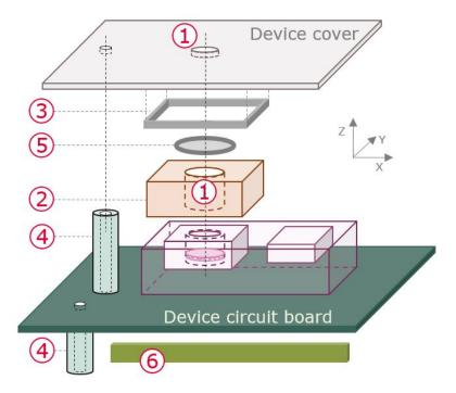
Figure 5 MEMS microphone mechanical design
