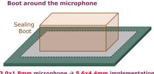
**3.0x1.8mm microphone**  $\rightarrow$  **5.6x4.4mm implementation** (with 0.8mm boot walls and 0.5mm clearance around the gasket)
