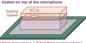
**4.0x3.0mm microphone**  $\rightarrow$  **5.0x4.0mm implementation** (with 0.5mm clearance around the microphone)
