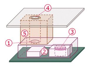
Figure 1 Microphone acoustic channel design
