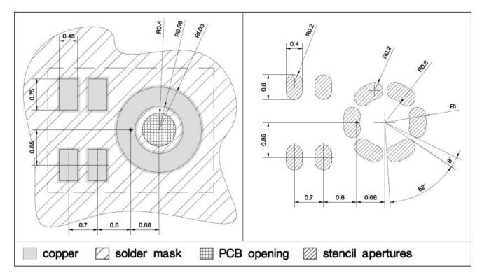
Figure 14 Infineon IM69D130 microphone footprint and stencil recommendation example
