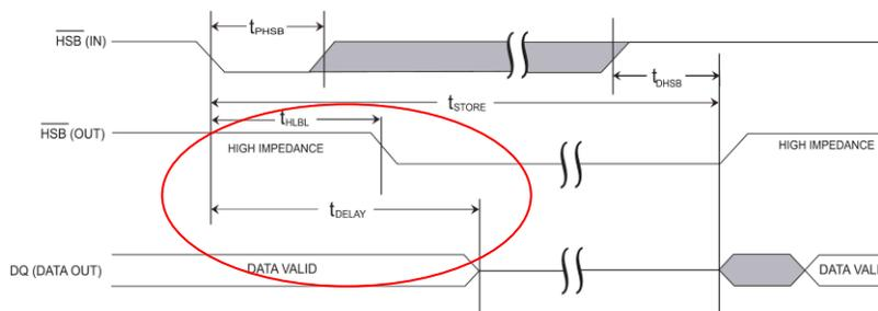
Figure 2. CY14E256LA: AC Parameters Related to  $\overline{HSB}$
