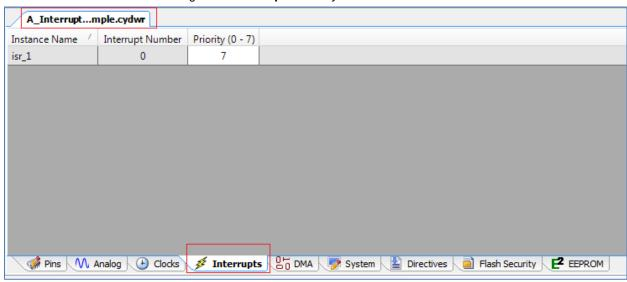
Use the *cydwr* window to change the priority of an interrupt. Remember that 0 has the highest priority, and 7, the lowest priority. The interrupt vector number for each Interrupt Component is automatically allocated by PSoC Creator when the project is built.
