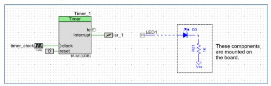
The Timer Component is a down counter, and the terminal count refers to the condition when the timer has reached its minimum value (zero). On the terminal count, the timer is reloaded with the period value and counting continues. An interrupt can be generated every time the terminal count condition occurs.
