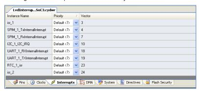
As mentioned in the previous section, you may need to override the vector numbers assigned by PSoC Creator and manually assign a vector number. A *Control File* is used to do this, as follows:
