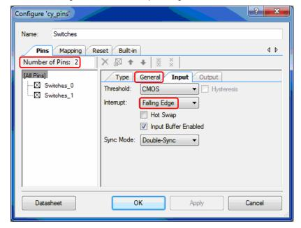
Figure 15. PICU Interrupt Configuration
