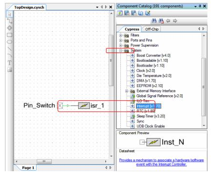
Figure 6. PSoC Creator Interrupt Component
