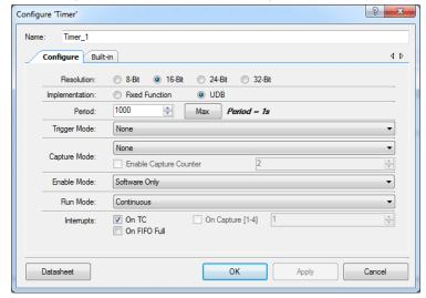
Figure 13. Timer Component Configuration
