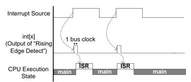
Figure 5. Edge Triggered UDB Interrupt Source
