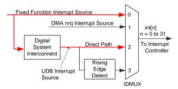
If the interrupt source is the DMA nrq signal, the dedicated path for the DMA nrq interrupt source is selected, as Figure 9 shows (see also Figure 4).
