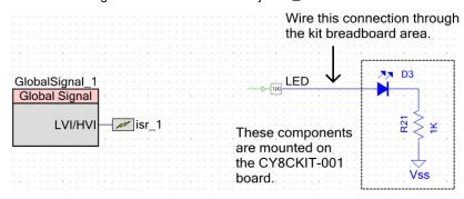
The Global Signal Reference Component makes it easy to use a number of system-level interrupts available in PSoC, as Figure 20 shows:
