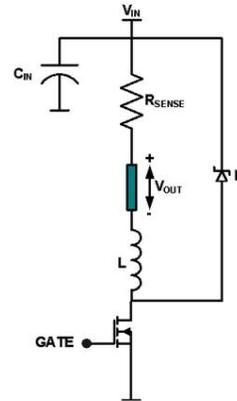
A floating load buck converter is a variant of buck topology, as shown in Figure 9. In such type of converters, capacitors across the output are usually not required, unless the current ripple is a contributing factor to EMI. When compared to a traditional buck topology, the switch is moved to the low side, the load is floating, and the diode is placed between the switch and the high side supply. The converter design equations are the same as that of a normal buck converter.
