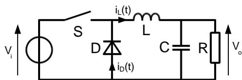
The buck converter, shown in Figure 1, is the simplest of all converters. A PWM signal of duty-cycle 'D' is used to drive the semiconductor switch 'S'. When the switch is on, the input voltage  $V_i$  is directly applied to one terminal of the inductor L. Assuming that the circuit has reached a steady state, the output voltage is at  $V_o$ . As a result, the voltage across the inductor is  $(V_i - V_o)$ . The inductor current is calculated using the following definition:
