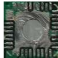
Figure 6. Good E-Pad Solder Mask (Reworked)
