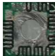
Figure 6. Good E-Pad Solder Mask (Reworked)
