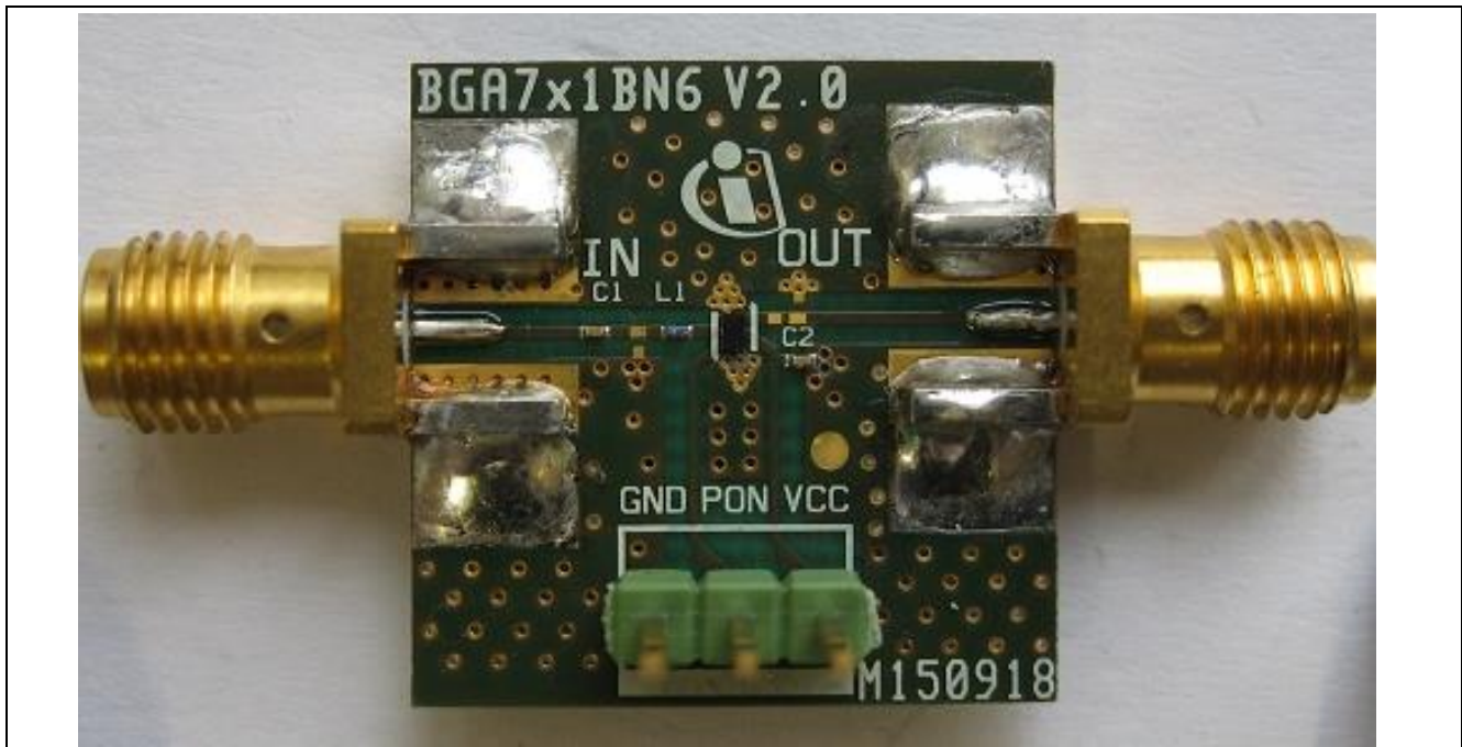
Figure 32 Photo Picture of Evaluation Board (overview) <PCB Marking M150918 Rev. 2.0>
